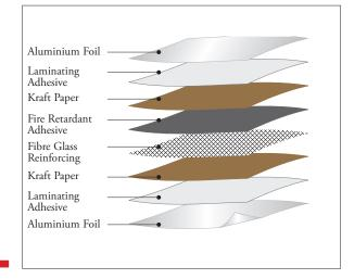
as an exposed internal roof lining. Thermofoil Medium Duty is suitable for these applications where high tensile strength and impact resistance is required.
